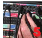
PATCH BAY Neal uses a Linux interface and SDI-routed cables to patch into the larger DreamWorks storage system.
