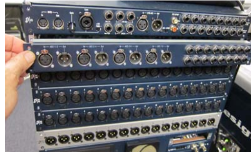
Sliding the IOx card into Slot A
