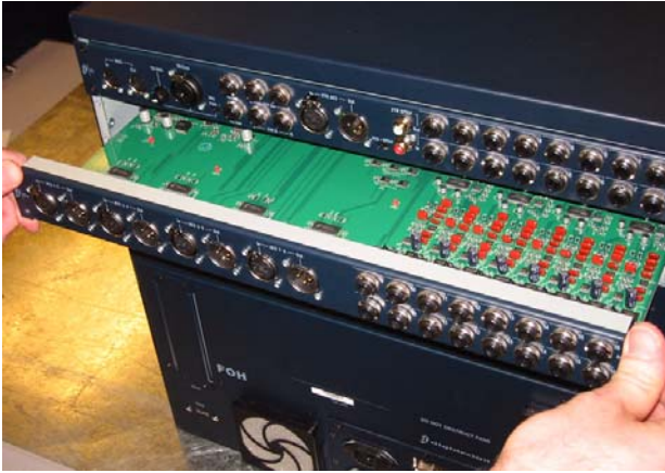
Installing the IOx card in the FOH Rack
